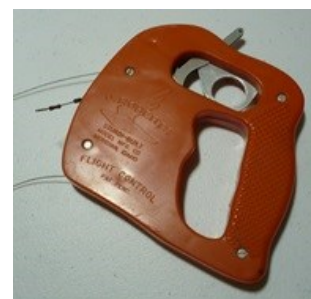
A plastic 3-Line reel with bell crank, "Sturdi-Built" by J. Roberts, made in Idaho.
